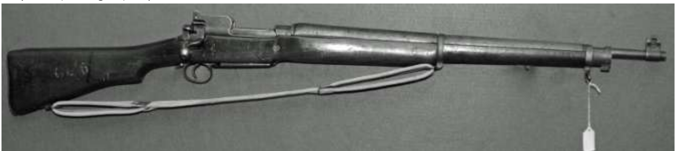
Eddystone Pattern 1914 rifle. The US produced the same rifle in 30.06 as the Rifle .30 cal Model 1917.
