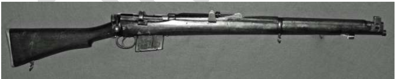
Rifle 7.62mm 2A1 (Indian 1964 on) – 7.62mm calibre, squared magazine and foresight protector ears. Shortened 1907 Bayonet
