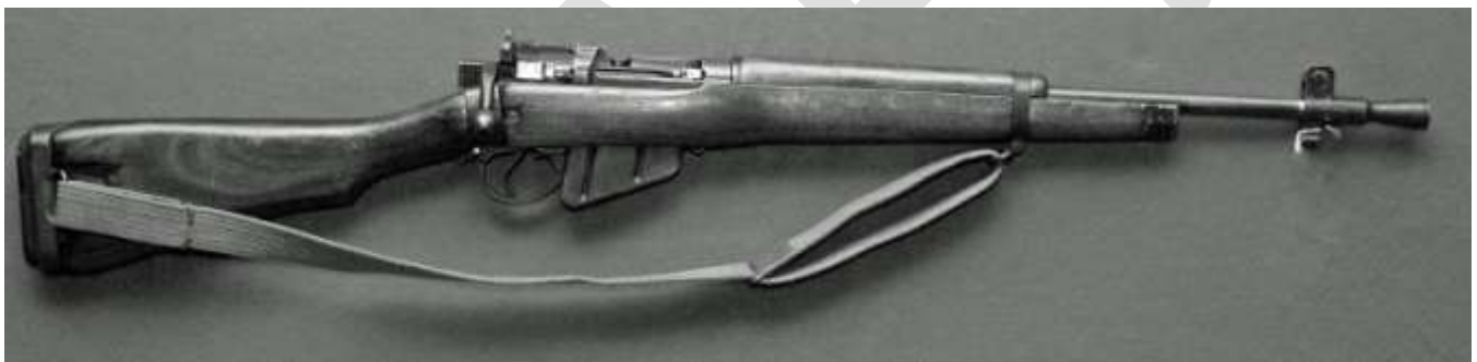
Lee-Enfield No5 Mk1 (WWII and on) – note flash hider, short length and receiver sight. Blade Bayonet
