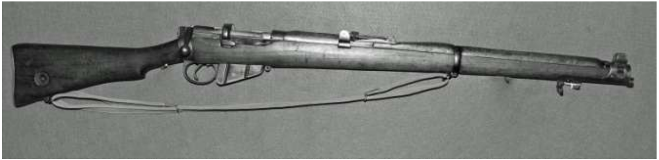
*Short, Magazine Lee Enfield MkIII* - simplified MkIII without volley sights, cut-off etc. P1903 / P1907 Bayonet
