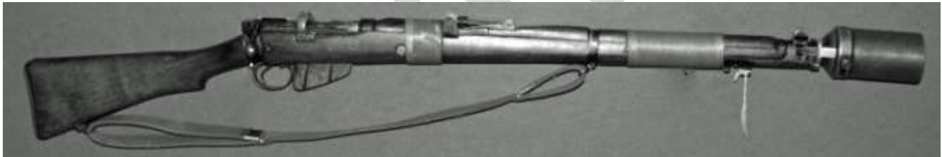
Grenade Launching Rifle (with cup discharger and wire wrap – see also the large transverse bolt behind rear wrapping)
